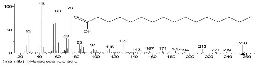
Fig 6 Mass spectrum of hexadecanoic acid
